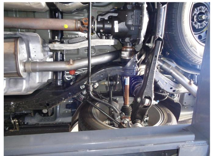
**Step 5.** If you have the MAX version of the Expedition you will need to loosely install the 11.25" Extension Pipe Assembly. Next, loosely attach the Over-Axle Pipe Assembly and the Tail Pipe Assembly using the supplied 3.00" clamps and engage the welded hangers to the OEM rubber insulators. Re-install sway bar.
