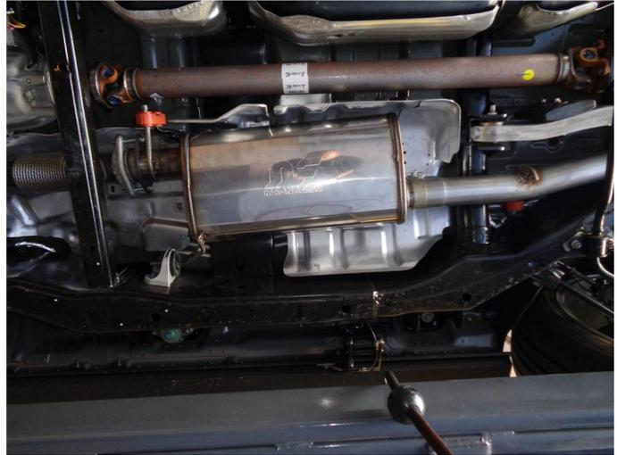
**Step 4.** Begin installing your new MAGNAFLOW system by loosely bolting the Muffer Assembly inlet flange to the flex assembly outlet using the supplied hardware.
