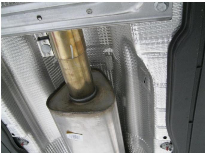
**Step 1.** Begin by loosening the factory clamp located just behind the catalytic converter. Working rearward extract the hangers from the rubber insulators (retain insulators as they will be used in the installation of the new exhaust system). Remove the OEM system from the vehicle.
