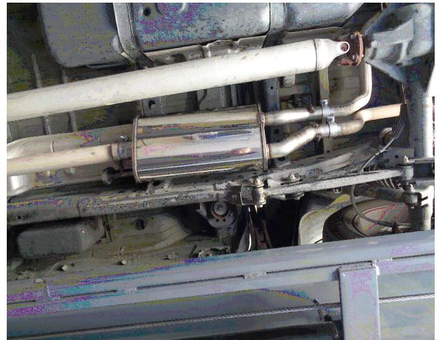
Step 4: Finish by fitting the OE tailpipes into the Muffler Assembly by indexing the alignment pegs and securing with the supplied 2.25" clamps. Once a final position has been chosen for the new exhaust system, evenly tighten all clamps from front to rear using the torque specifications on page one of these instructions. Inspect all fasteners after 25-50 miles for operation and re-tighten if necessary.
