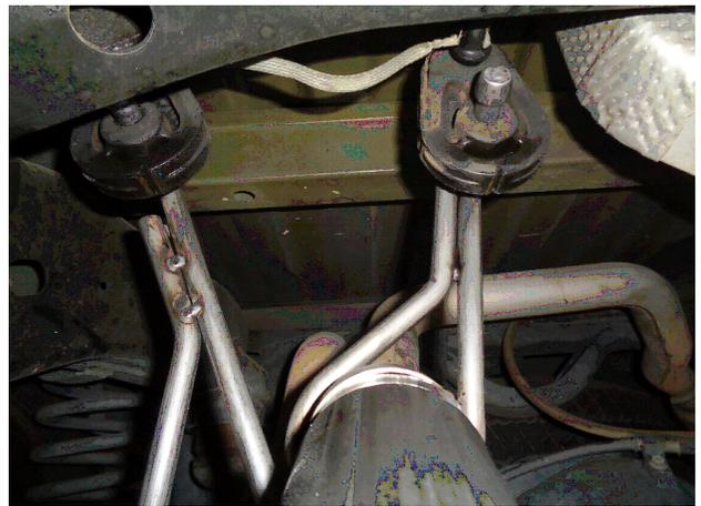
Step 3: insert the welded hangers into the rubber insulators
