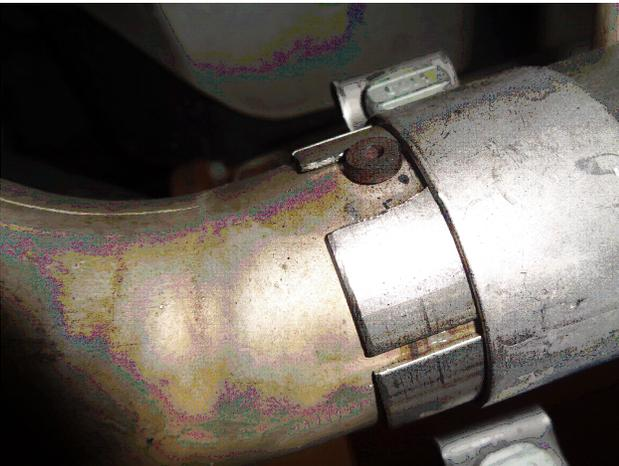
Step 2: To install the MagnaFlow Muffler Assembly slide the inlet onto the OE outlet making sure to align the slot with the peg on the outlet pipe. Secure with the supplied 3.00" clamp.
