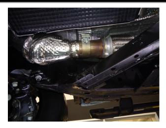
Step 2. Begin installation by attaching the Inlet Pipe Assembly to the outlet of the catalytic converter using the supplied 2.50" clamp and fitting the welded hanger into the rubber insulator (Leave all clamps and fasteners loose for final adjustment of the complete system.)
