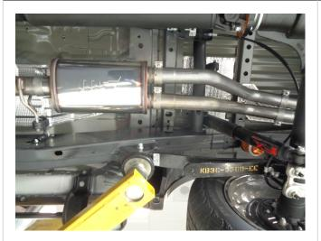
Step 4. Attach the Driver and Passenger Over Axle Pipes to the Muffler Assembly using the supplied 2.50" clamps and engaging the welded hanger.
