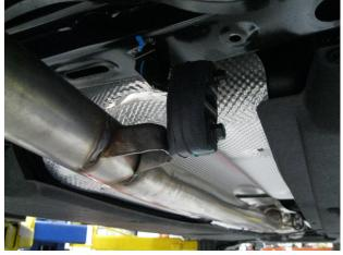
Step 1. To extract the OEM exhaust system begin by un-fastening the flange located behind the catalytic converter and the second flange located in front of the Driver side muffler assembly. Next, working rearward, disengage all welded hangers from the rubber insulators. Do not damage or discard the rubber insulators or fasteners as they will be re-used to mount the new system. You can now remove the exhaust from the vehicle.
