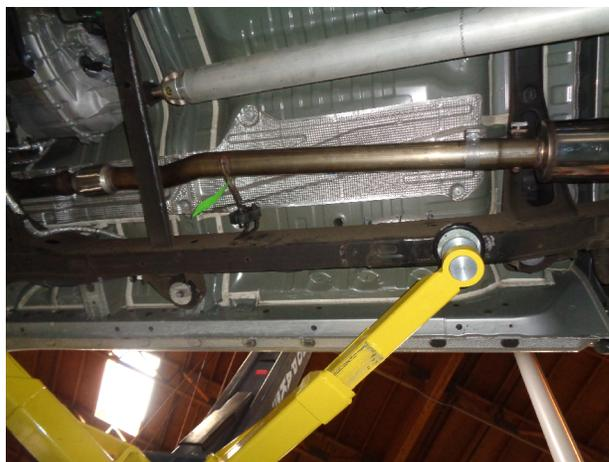
**Step 3.** Install the appropriate extension pipe depending on the cab size. Install the Inlet Pipe using the supplied 3.00" clamp then attach the Muffler Assembly to the Extension Pipe.
