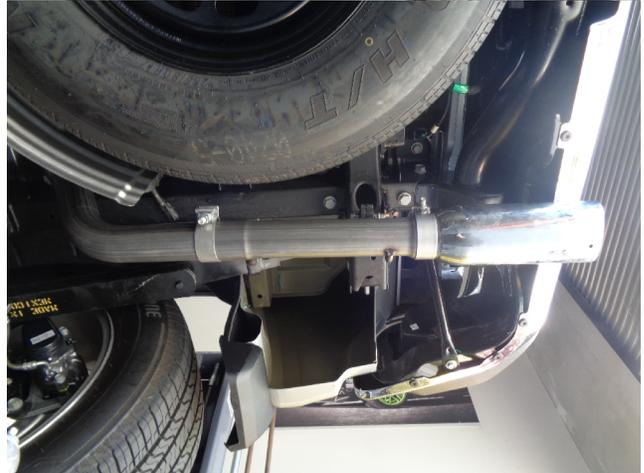
**Step 6.** Using the supplied rubber insulators install the Tailpipe Assemblies to the Extension pipes fitting the hangers into the installed hanger brackets.
