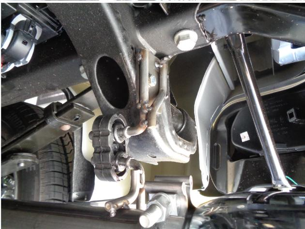
**Step 5.** As this vehicle was not setup for dual exhaust from the factory, hanger brackets will need to be installed. Install the hanger brackets on the rear frame section using the supplied fastener hardware as shown
