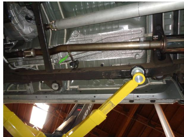
**Step 3.** Only the Crew Cab Long Bed configuration will require the supplied 12.5 Extension Pipe, Install this to Inlet Pipe Assembly if required using the supplied 3.00" clamp then attach the Muffler Assembly to the Extension Pipe. If the 12.5" Extension Pipe isn't used attach the Muffler Assembly directly to the Inlet Assembly with a supplied 3.00" clamp.
