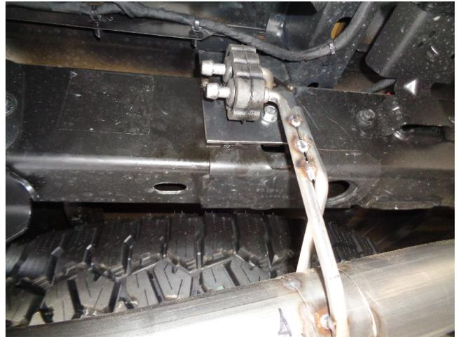
**Step 5.** As this vehicle was not setup for dual exhaust from the factory, a hanger bracket will need to be installed to the frame on the Passenger side with the supplied hardware as shown. Use the supplied zip tie to move the breather tube out of the way.
