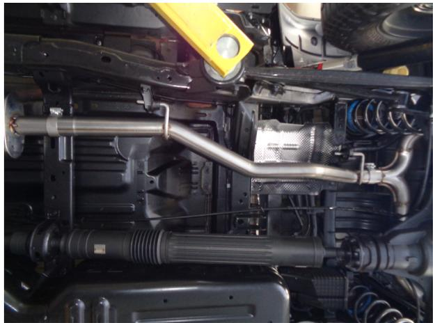
**Step 3.** Install this to the Inlet Pipe Assembly using the supplied 3.00" clamp and attaching the hangers, then attach the Y-Pipe Assembly to the Extension Pipe.
