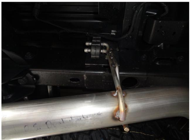
**Step 6.** Next loosley attach the Passenger Side Tailpipe to the Y-Pipe by using the hanger brackets and the supplied 2.50" clamp.
