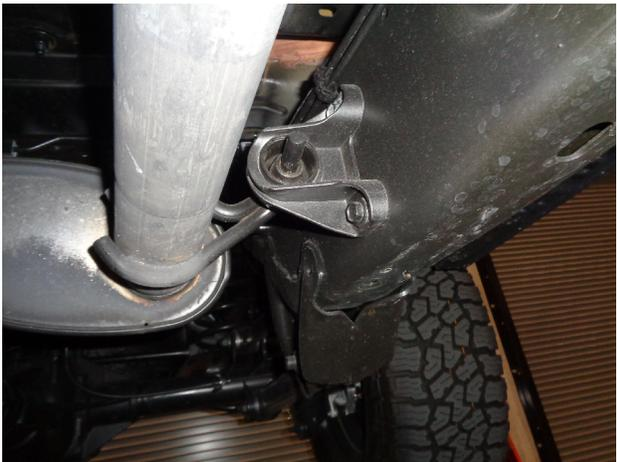
**Step 1.** To remove the OEM exhaust system, you will need to remove the spare tire first. You can then disengage the welded hangers from the rubber insulators and remove the tailpipe assy. Unfasten the clamp attaching the OEM inlet pipe assembly to the catalytic converter. Do not damage or discard the inlet pipe clamp or rubber insulators as they will be re-used to mount the new system. Disengage the inlet pipe assembly hanger and remove the exhaust from the vehicle.
