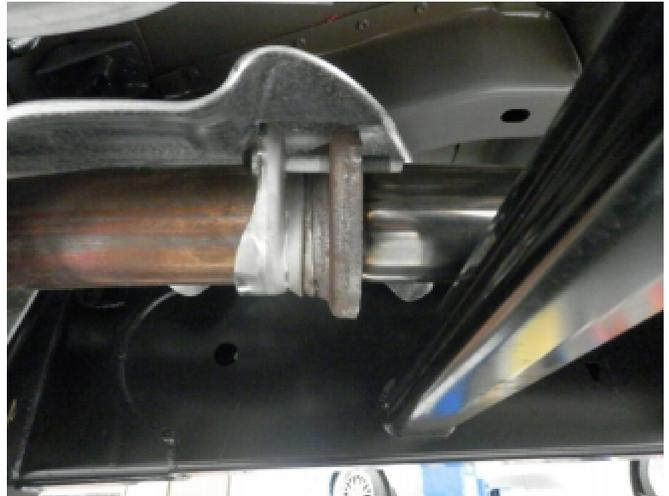
Step 4. Before installing the Muffler Assembly there is an OEM rubber insulator assembly bolted to the subframe that may need to be removed before installing the Muffler Assembly. If your vehicles engine is 2.7L or 3.5L you will need to remove the rubber insulator assembly. If you have the 5.0L leave the rubber insulator intact.
