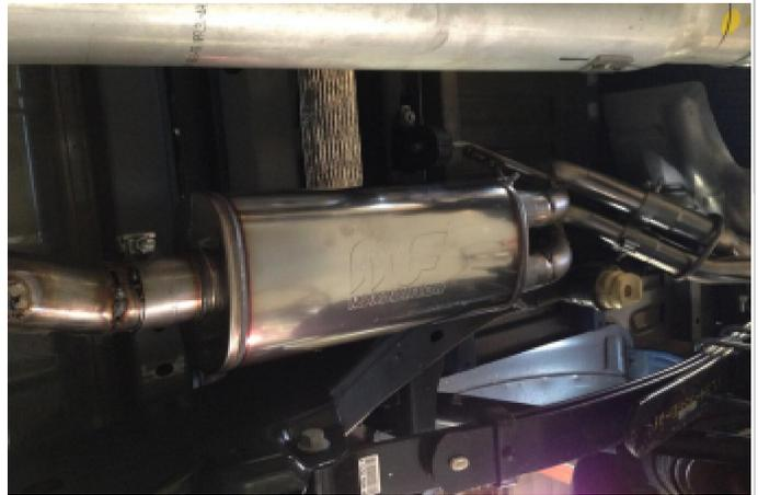
Step 3. Install the Muffler Assembly to the Inlet Pipe Assembly using the supplied 3.00" clamp.
