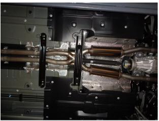
**Step 2.** Begin installation of the new system by attaching the Driver and Passenger side (Passenger is the longer of the two pipes) inlet pipes to the outlets of the OEM system using the supplied 2.25" clamps. Next attach the Resonator Assembly to the inlet pipes with supplied clamps and insert the hangers into the rubber insulators.
