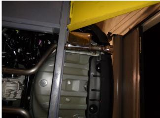
**Step 3.** Attach the Muffler Assemblies to the Resonator Assembly with supplied 2.50 Clamps and aligning them with the openings in the rear valance. Fit hangers into rubber insulators. Remember to reattach the ground strap to the hanger. Finish the installation by mounting underbody braces.
