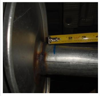
Step 2. Next cut the exhaust rearward of the muffler 0.5" behind the welded the muffler. Disengage the welded hanger on the muffler from the rubber insulators. Remove the muffler section. Deburr the sharp edges from the cut ends. You are now ready to install your new MAGNAFLOW system.
