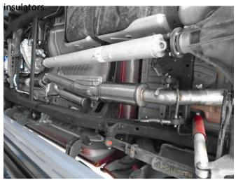
Step 6. With the new MAGNAFLOW system in place all loose band clamps can now be tightened. Your installation is complete.
