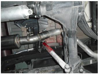
Step 5. Slip the Outlet Resonator exit pipe over the cut OEM rear pipe. Loosely secure using the supplied band clamp. Engage the welded hangers to the rubber
