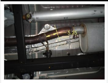
Step 1. The muffler section will need to be removed from the OEM exhaust system. Using a Sawzall or similar cutting tool cut the exhaust pipe 5.25" rearward of the welded hanger in front of the muffler.
