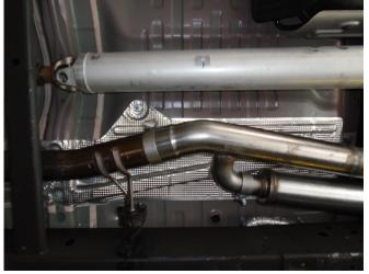
Step 3. Begin installation by slipping the inlet of the Inlet Resonator Assembly over the cut OEM outlet pipe. Secure using the supplied band clamp. Keep all clamps loose until the final assembly is complete to
