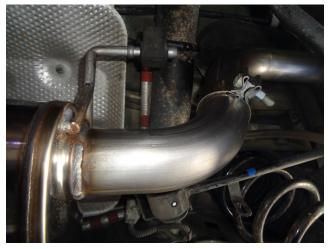
Next, attach the Overaxle pipe to the muffler Assembly and loosely tighten.
