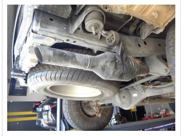
Working front to rear disengage all welded hangers from the rubber insulators and remove the system. (Retain the insulators as they will be needed to mount the new MAGNAFLOW system.)
