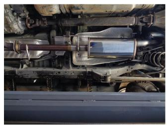
**Step 3:** Install the new system by attaching inlet pipe and muffler assembly with the supplied hardware.
