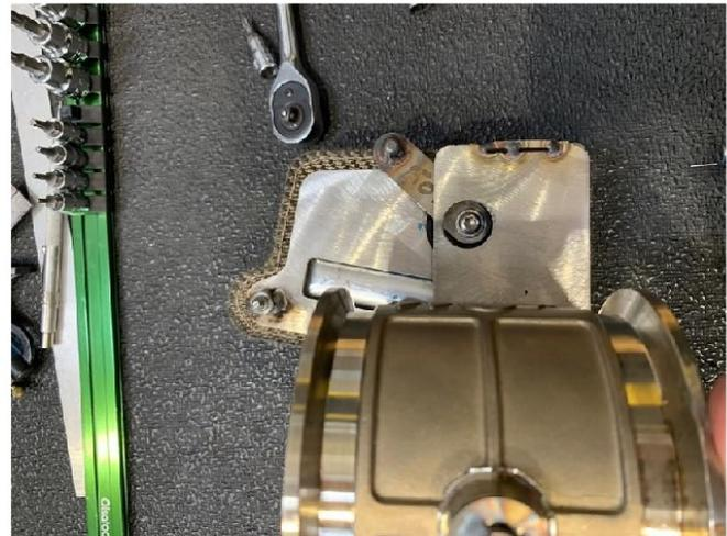
**Step 21.** Attach the MF control arm to the OE valve motor as shown using the remaining OE screw.
