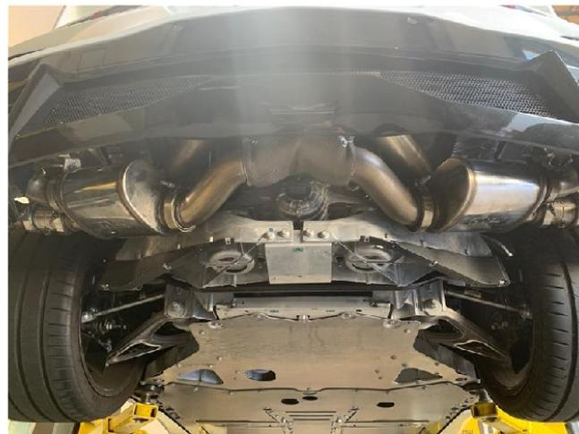
**Step 30.** Loosely install both Muffler/Tip assemblies to the X-Pipe Assembly. Loosely secure using the supplied clamps. Engage the welded hangers to the rubber insulators.
