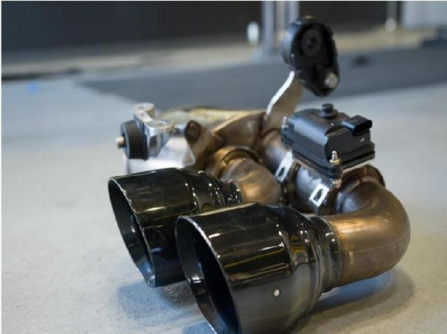
**Step 28.** Place the supplied valve gasket between each valve and valve motor. Secure the OE valve motors to both Muffler/Tip Assemblies using the OE hardware.
