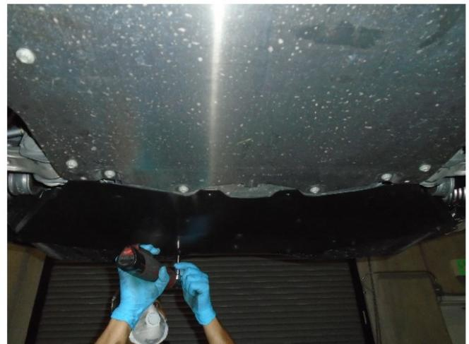
**Step 6.** Next remove the rear sub-frame underside cover by removing (11) 7mm hex head screw and (1) push pin clip.
