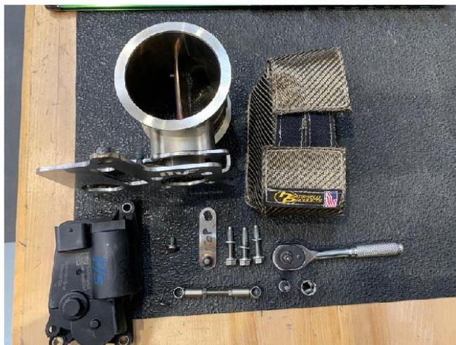
**Step 19.** Account for the parts you will need to assemble the Inlet Valve assembly. MF 3.00" Valve, OE Valve Motor, OE Adjustable control arm, MF control arm, MF Heat Blanket and [4] OE screws.
