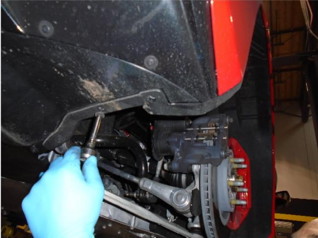
**Step 1.** Remove the OEM system by first removing both rear wheels. Next remove the wheel well covering by removing (5) 7mm hex head screws forward and rearward of the wheel well.
