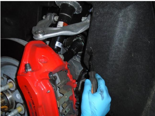
**Step 3.** Remove the 4 push pin clips attaching the wheel well liner.
