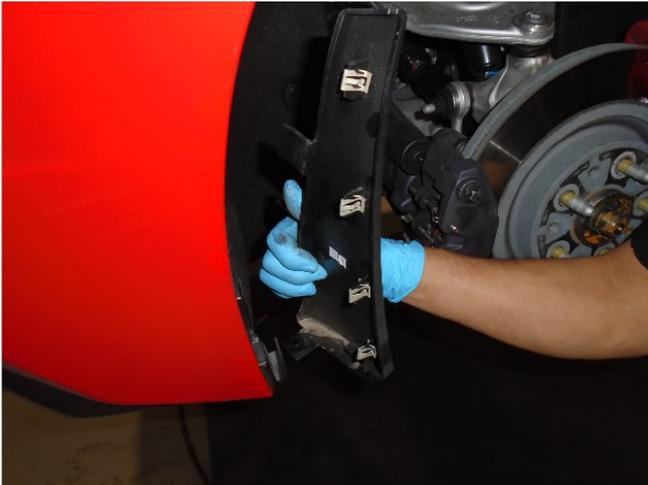
**Step 2.** Remove the Splash Guard Trim by gently pulling to release the retaining clips.
