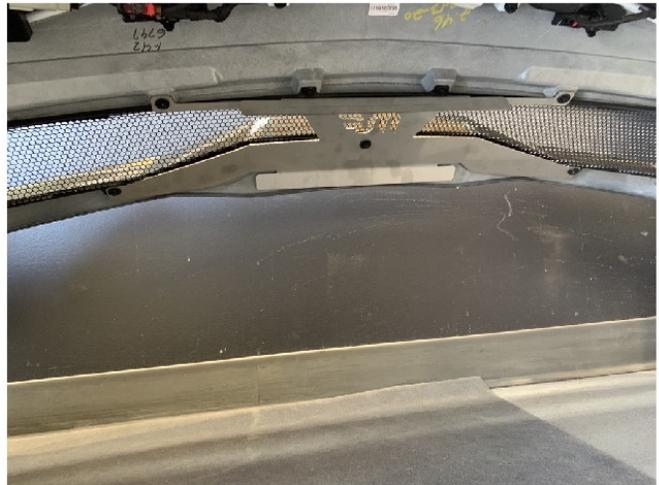
**Step 30.** Install the Rear Fascia Heat Shield by removing [4] bolts attaching the mesh. Locate the holes in the heat shield and secure using the OE screws.
