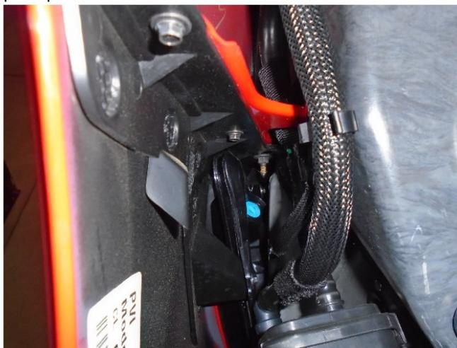
**Step 8.** The bumper and rear valance must be removed together. First remove the 10mm nut attached to the smog pump on the passengers side of the vehicle.
