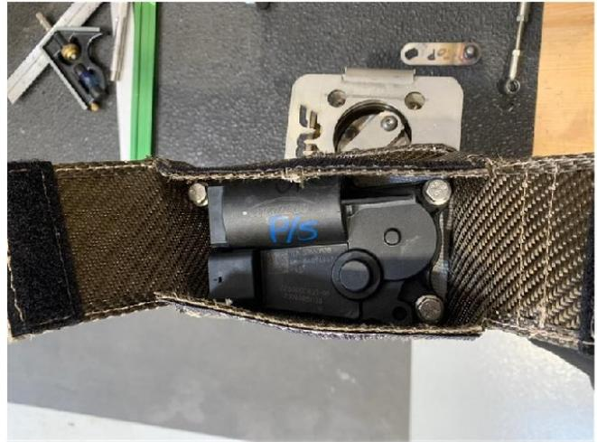
**Step 20.** Place the OE valve motor into the MF valve heat blanket as shown. Align the three holes in the motor, heat blanket and valve top plate. Secure using the three OE screws.
