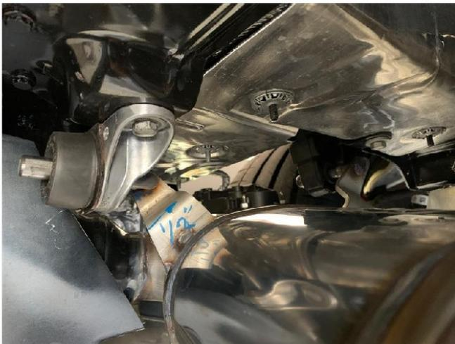
**Step 29.** Reattach both hanger brackets with the OE hardware.
