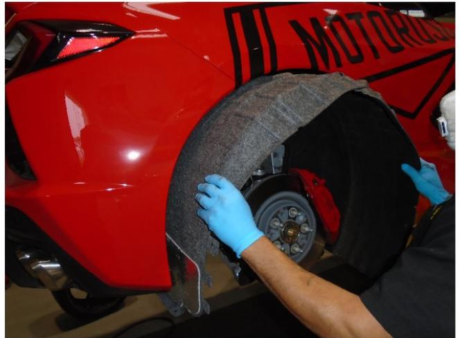
**Step 5.** The wheel well trim can now be removed. Duplicate the process for the other side.
