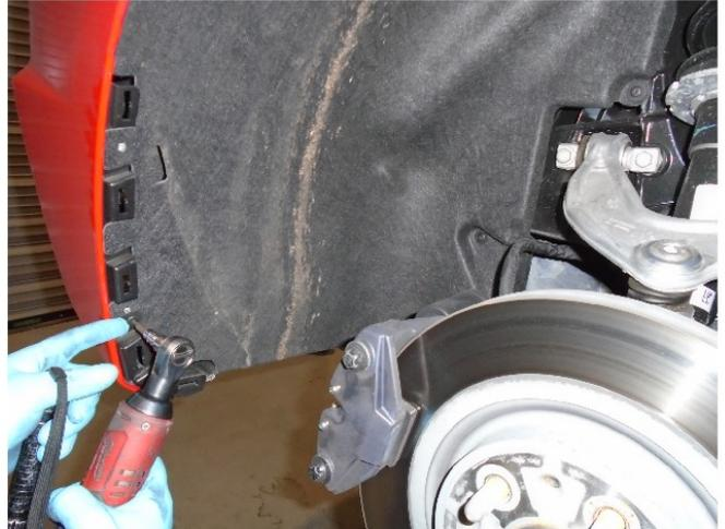
**Step 4.** Remove (11) T-15 Torx head screws securing the wheel well trim.
