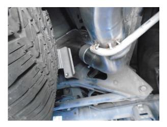
Next, loosely attach the Mid-Pipe to the muffler outlet using a supplied 2.50" clamp.
