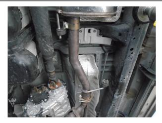
**Step 2:** Begin Installing the new system by attaching the inlet pipe to the Catalytic Converter outlet using the OE spring bolts.
