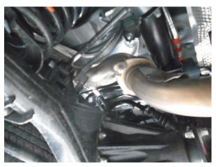
**Step 1:** To remove the OE exhaust system begin by unfastening the two bolt spring fasteners towards the front of the vehicle, moving front to rear loosen the clamps and fasteners at the pipe junction points. disengage all welded hangers from the rubber insulators and remove the system. (Retain the rubber insulators and inlet spring bolt fasteners as they will be used to mount the new MagnaFlow system.)
