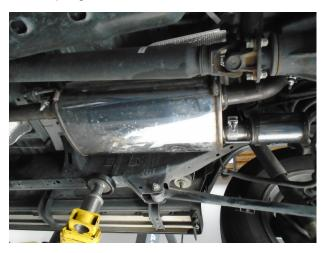
**Step 3:** Next attach the Oval Muffler to the Inlet Pipe with the supplied 2.50" clamp. This exhaust system is configured to allow the user to tune the sound. For a more moderate exhaust tone install the  $4.00 \times .6.00$ " NDT (No Drone Technology) Chamber (as shown) using the suppled 2.50" clamps. For a more aggressive sound block the Muffler outlet with the supplied MF logo'd cap.
