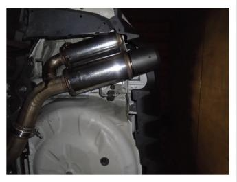
**Step 5**. Complete the installation by mounting the Muffler NDT Assembly to the Mid Pipe using the supplied clamp and inserting the hangers into the rubber insulators.
