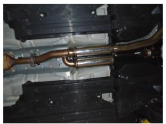
**Step 4**. Begin assembly of the new MagnaFlow system by attaching the Inlet NDT Resonator Assembly to the catalytic convert outlet using the OE fasteners. Next you will need to determine the tone you want for your vehicle, install the 14x4" Mid Resonator or the xTREME Delete using the supplied 3.00" Clamp. (leave all clamps and fasteners loose until final positioning of the complete system.)
