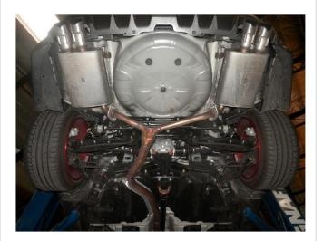
**Step 2**. Next, remove both muffler assemblies by unfastening them from the OE Y-Pipe and extract the welded hangers from the rubber (Retain all mounting hardware and rubber insulators as they will be used to install your new MagnaFlow system.)
