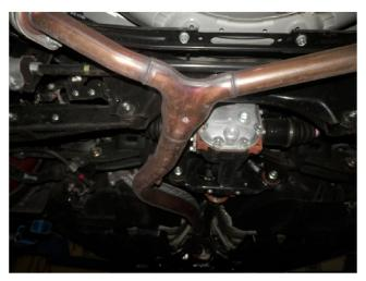
**Step 3**. Finish dis-assembly by removing the remaining hanger from the rubber insulator and removing the Y-Pipe.
