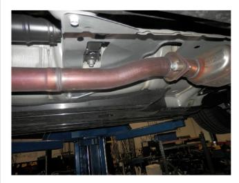
**Step 1**. Begin removal of the OE exhaust system by unfastening the 2 bolt flange at the catalytic converter.
