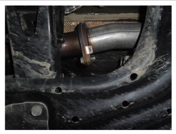
**Step 1:** Begin removal of your OE system by first removing the nuts at both inlet flange junctions.
