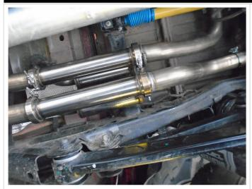
Step 5: MagnaFlow supplies this kit with multiple build options giving the ability to use different muffler, NDT and muffler deletes depending on preference.
