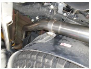
**Step 7:** Loosly install the two Tailpipe Extension Pipes using the supplied clamps. The longer, three bend pipe will be for the drivers side.
