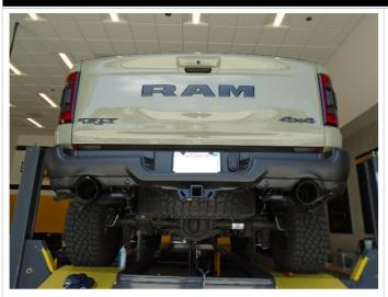
**Step 9:** Once a final position has been chosen for the new exhaust system, evenly tighten all clamps and fasteneners, from front to rear, using the torque specifications on page one of the instructions. Inspect all fasteners after 25-50 miles of operation and re-tighten if necessary.
