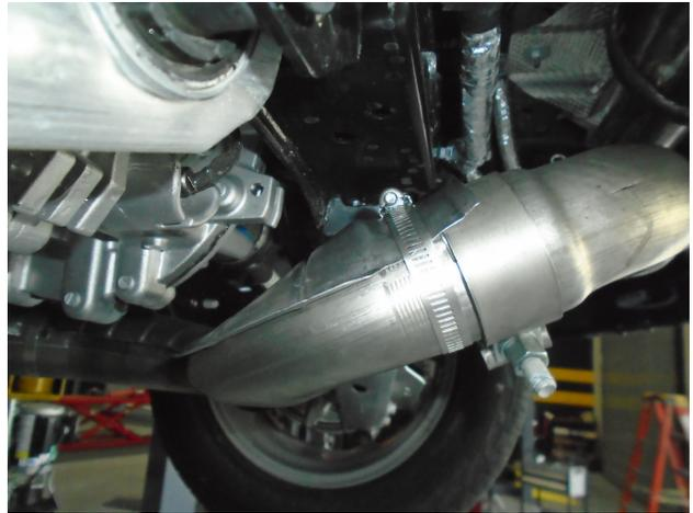
**Step 2:** Begin installing the new exhaust system by attaching the specific Inlet Pipe (2.0L or 1.5L engine) to the cut OE outlet using the supplied 2.18/2.36 clamp. Use the supplied hose clamp to re-attach the heatshield if necessary.
