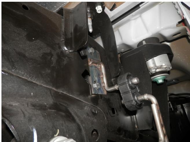
**Step 5.** Locate the two square holes in the passengers side of the vehicles subframe. Attach the two supplied U-Type panel nuts as shown in the diagram. Losely bolt the supplied Hanger Bracket Assembly to the panel nuts using the supplied bolts.
