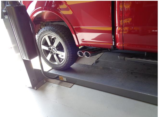
**Step 7.** Once a final position has been chosen for the new exhaust system, evenly tighten all clamps from front to rear using the torque specifications on page one of these instructions. Inspect all fasteners after 25-50 miles of operation and re-tighten if necessary.
