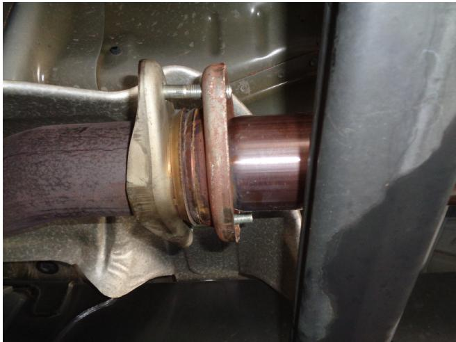
**Step 1.** To remove the OEM exhaust system, you will need to unbolt the muffler assembly from the flange junction as shown.
