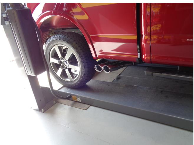
**Step 7.** Once a final position have been choden for the new exhaust system, evenly tighten all clamps from front to rear using the torque specifications on page one of these instructions. Inspect all fasteners after 25-50 miles if operation and re-tighten if necessary.
