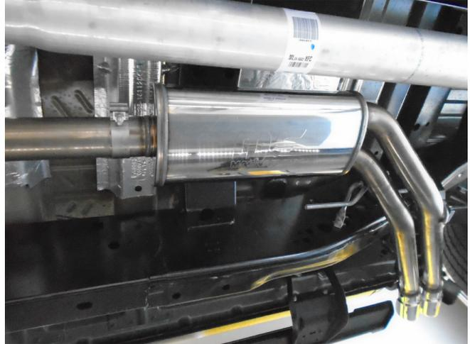
**Step 6.** Install the Muffler Assembly and loosely secure using the supplied 3.00" clamp. Attach the installed Hanger Bracket Assembly to the welded hanger using the supplied rubber insulator.
