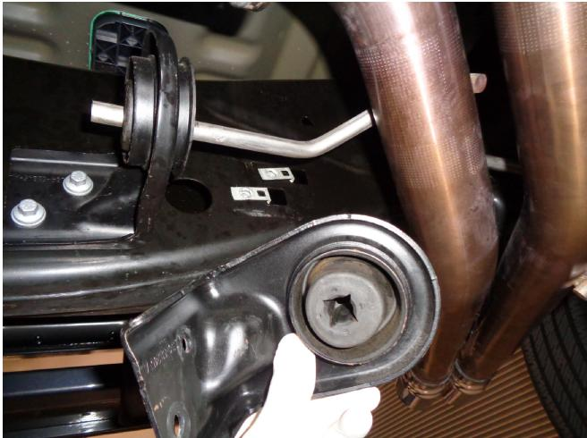
**Step 4.** Before installing the Muffler Assembly there is an OEM rubber insulator assembly bolted to the subframe that may need to be removed before installing the Muffler Assembly. If your vehicles engine is 2.7L or 3.5L you will need to remove teh rubber insulator assembly. If you have the 5.0L leave the rubber insulator intact.
