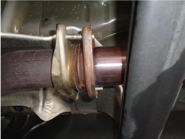
**Step 1.** To remove the OEM exhaust system, you will need to unbolt the muffer assembly from the flange junction as shown.
