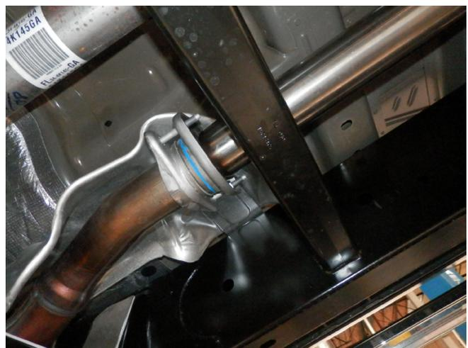
**Step 3.** Your new MAGNAFLOW system comes with two inlet pipe assemblies. The assembly that has the flange welded to it is for year spread 2015 - 2020. The pipe without the flange will use the slip flange in the hardware kit and is for years 2021. Loosely attach the correct pipe assembly for your year of vehicle using either the OE hardware or the supplied hardware.
