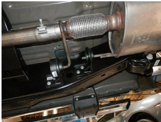
**Step 2.** Unbolt the clamp just behind the muffer. Disengage the welded hangers from the rubber insulators. Remove the OEM exhaust system. Do not damage or discard the OEM fasteners or rubber insulators as they will be reused to mount your new MAGNAFLOW system.
