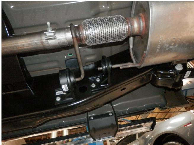
**Step 2.** Unbolt the clamp just behind the muffler. Disengage the welded hangers from the rubber insulators. Remove the OEM exhaust system. Do not damage or discard the OEM fasteners or rubber insulators as they will be reused to mount your new MAGNAFLOW system.
