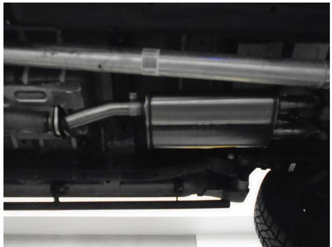
**Step 5:** Next attach the Oval Muffler to the Inlet Pipe with the supplied 2.50" clamp. This exhaust system is configured to allow the user to tune the sound. For a more moderate exhaust sound install the U-pipe Assy and the 4.00" NDT Chamber (as shown) using the supplied 2.50" clamps. For a more aggressive sound see configuration chart below.
