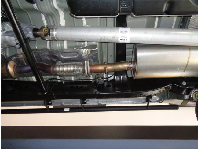
**Step 1:** To remove the OEM exhaust system, unfasten hardware at the muffler flange (Retain both flange fasteners to be re-used).
