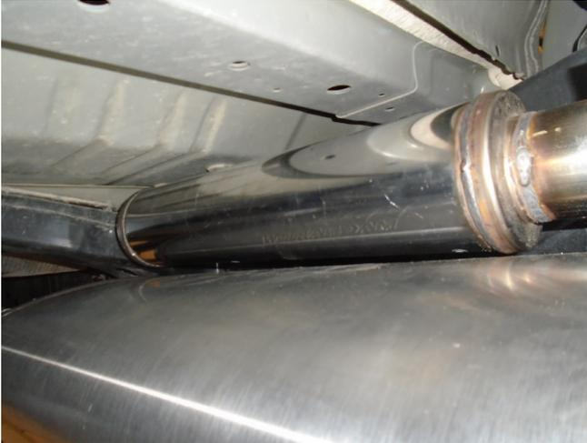
When using the NDT chamber, mount it above the muffler as shown. Be sure to leave at least 1/2" of clearance between both components.
