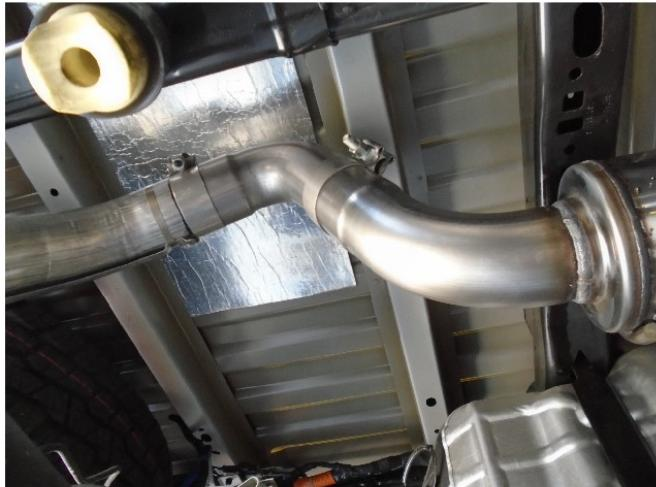
**Step 7:** For 2021 models slip the Muffler Assembly outlet to the supplied Outlet Pipe with the 3" clamp. Then attach the cut tail pipe using the 3.18" clamp. Loosely secure both clamps.
