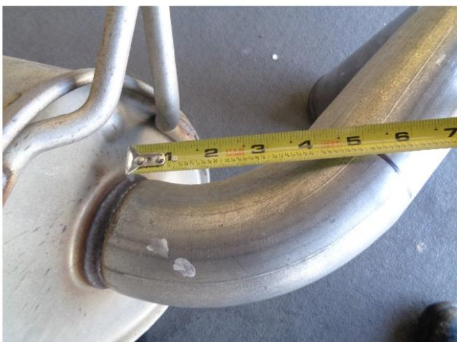
**Step 1.** For '15-'20 models begin removal of the OE muffler by marking cut point to the rear of OE Muffler as shown in photo below. Then cut the OE Exhaust at that cut point.
