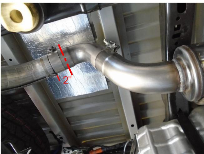
**Step 2.** For 2021 cut the 2" forward of the OE tail pipe heat shield.
