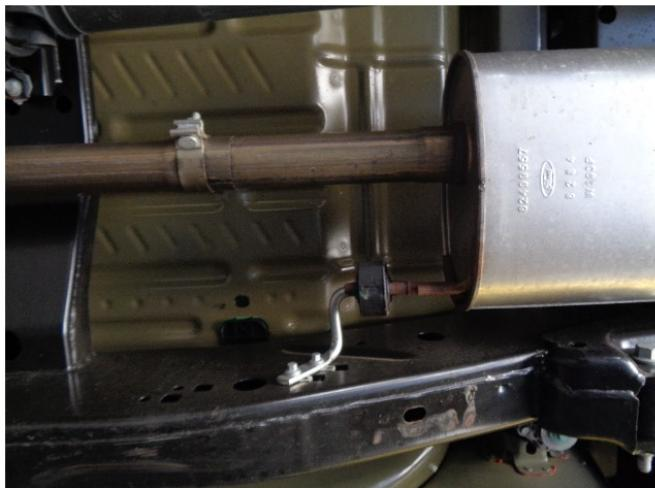
**Step 3:** Remove the mid section of the OE exhaust by loosening the clamp forward of the muffler shown. Then disengage the hangers from the rubber insulators. Be sure to not damage the rubber insulators as these will be used for the new MAGNAFLOW Muffler.
