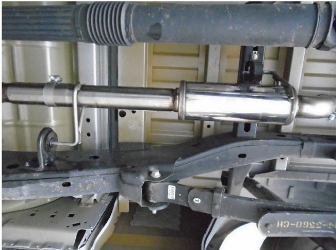
**Step 5:** Slip the Muffler Assembly inlet over the Inlet Pipe outlet. Loosely secure with the supplied clamp. Engage the welded hangers to the rubber insulators.
