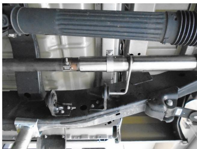
**Step 4:** Install Inlet Pipe for your application. The smaller inlet diameter is for 2015 - 2020, the larger is for 2021. Loosely attach the inlet of the Inlet Pipe to the vehicles inlet pipe outlet using the OE clamp.
