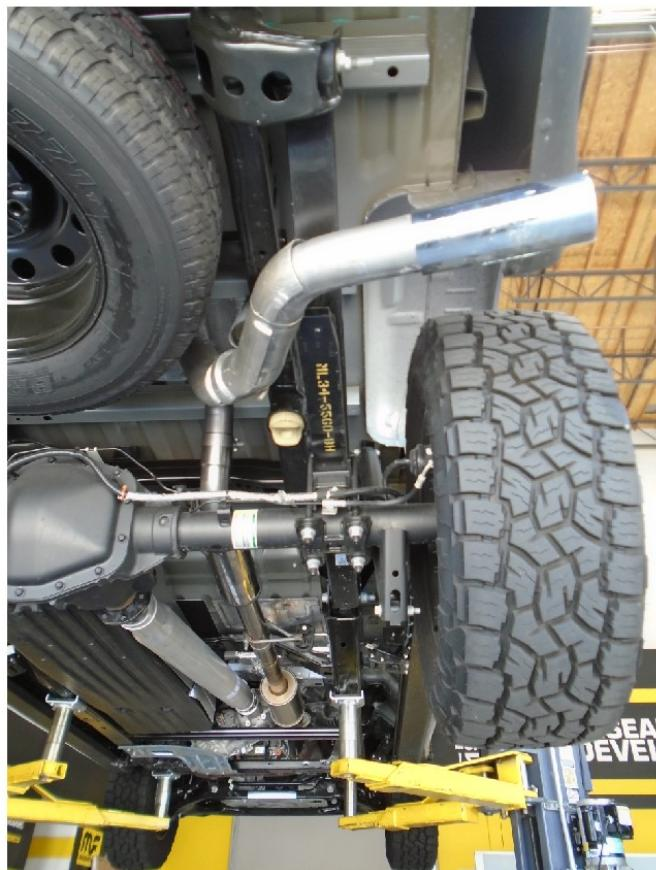
**Step 8:** Once a final position has been chosen for the new exhaust system, evenly tighten all clamps. Inspect after 25-50 miles for operation and re-tighten if necessary.
