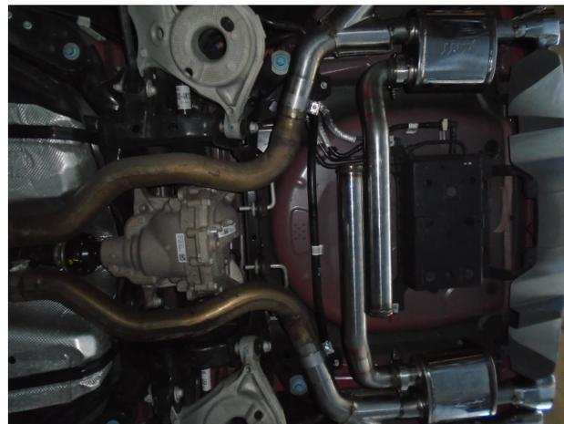
**Step 3.** Next attach the Mid Pipe Assemblies to the X-Pipe using the supplied 3.00" clamps and fitting the hangers into the rubber insulators.
