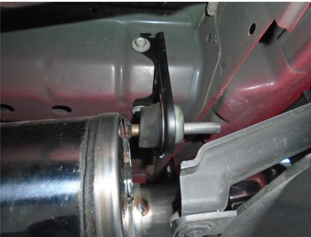
**Step 4.** Next install the passenger side NDT Muffler Assembly followed by the driver side NDT Muffler Assembly using supplied 3.00 Band Clamps and engaging the hangers into the rubber insulators.
