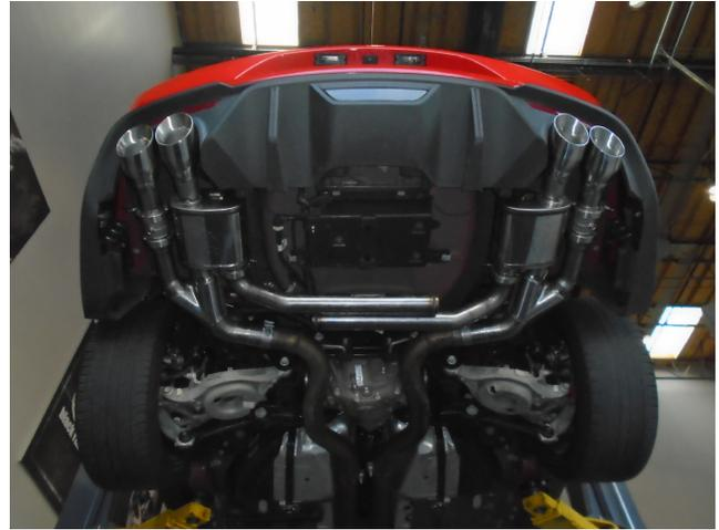
**Step 5.** Finish by installing the NDT Resonator Assemblies using the supplied 2.50" V clamps and rotating so they are level or horizontal to the ground. It is critical that the NDT Resonators are not in close proximity to moving suspension, plastics, or electronics as they can get extremely hot.
