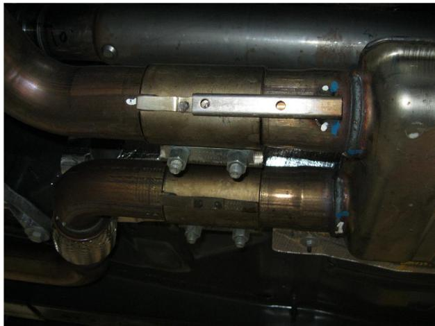
**Step 1.** Remove the OE exhaust system by first loosening the clamps located in front of the resonator. Next working front to rear extract the hangers from the rubber insulators and remove the complete exhaust system. Retain insulators and clamps as they will be used to install the new system.
