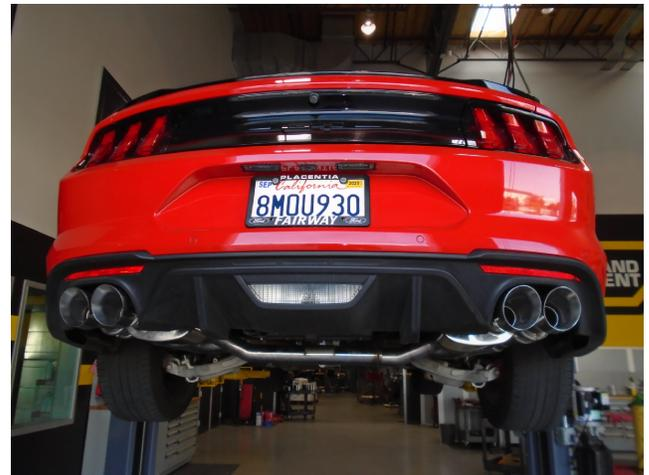
**Step 6.** Once a final position has been chosen for the new exhaust system, evenly tighten all clamps and fasteners using the torque specifications on page one of the instructions. Inspect all fasteners after 25-50 miles of operation and re-tighten as necessary.
