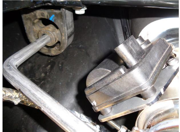
**Step 5.** If your vehicle has valves re-connect the wiring harness plugs to the Valve motors, re-install the rear valance.
