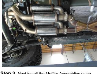
**Step 3.** Next install the Muffler Assemblies using the supplied V-Band clamps. Fit the hanger on the driver side assembly into the rubber insualtor.
