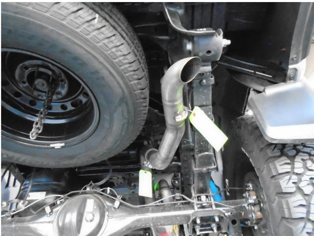
**Step 6:** Finish by installing the Tail Pipe Assembly to the Over Axle Assembly using the supplied 2.50" clamp and OE rubber insulator
