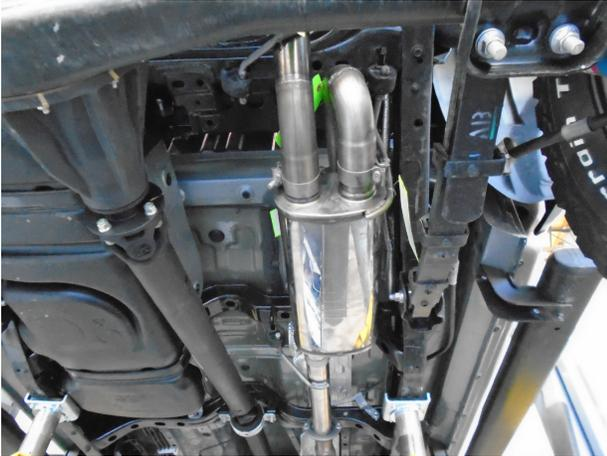
**Step 5:** Attach the Over Axle Pipe to the Muffler Assembly as shown using the provided 2.50" clamp and the OE rubber insulator.
