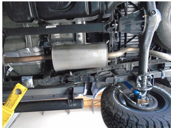
**Step 2:** Working front to rear, disengage all welded hangers from the rubber insulators and remove the system. (Retain the rubber insulators as they will be needed to mount the new MagnaFlow system.)
