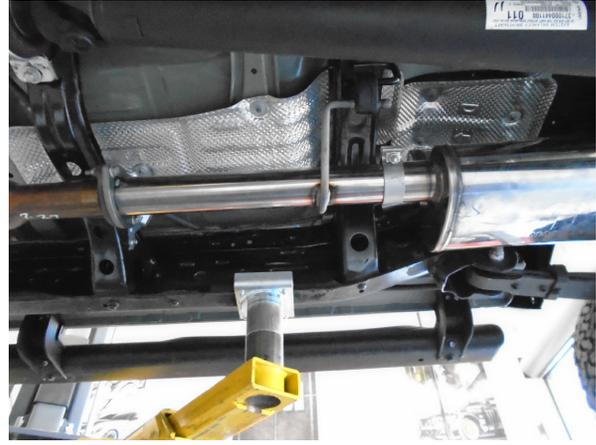
**Step 3:** Begin Installing the new system by attaching the inlet pipe to the vehicle using the OE Fasteners. and engaging the hanger into the rubber insulator.
