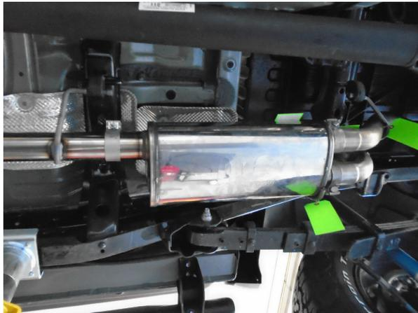
**Step 4:** Next attach the Oval Muffler to the Inlet Pipe with the supplied 2.50" clamp. This exhaust system is configured to allow the user to tune the sound. For a more moderate exhaust sound install the U-pipe Assy and the 4.00" NDT Chamber (as shown) using the supplied 2.50" clamps. For a more aggressive sound see configuration chart below.
