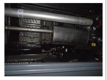
**Step 2.** Remove the OE inlet muffler assembly by loosening the band clamp on the inlet pipe. Remove the inlet muffler asembly. You are now ready to install your new MAGNAFLOW exhaust system.
