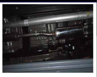
**Step 3.** Begin the installation by loosely attaching the Muffler Assembly to the outlet using the OE clamp and fitting the hanger into the rubber insulator.
