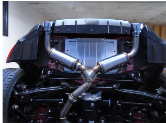
**Step 4.** Install the Muffler Assemblies in a similar fashion using the supplied 2.50" V-clamps and fitting the hangers into the insulators.
