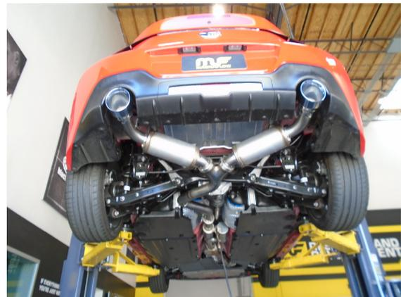
**Step 5.** Once a final position has been chosen for the new exhaust system, evenly tighten all clamps from front to rear using the torque specification on page one of these instructions. Inspect all fasteners after 25-50 miles of operation. Re-tighten if necessary.
