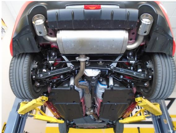
**Step 1.** Begin removal of your OEM exhaust system by unbolting the flange behind the catalytic converter. Remove all welded hangers from the rubber insulators. The exhaust can now be removed. Retain all fasteners and insulators as they will be needed to mount your new MagnaFlow exhaust system
