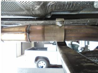
**Step 2.** Begin installation of the MagnaFlow system by attaching the X-Pipe Assembly with the supplied 2.75" clamps and fitting the hanger into the rubber insulator (Leave all clamps loose for final adjustment of the complete system.)
