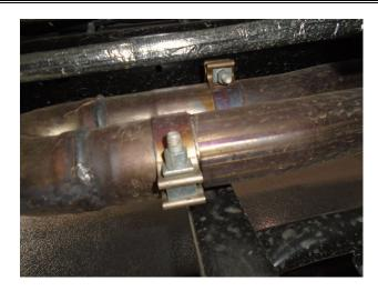
**Step 1.** Remove the OE system by loosening the clamps at the exhaust inlet. Extract the welded hangers from the rubber insulators remove the vacuum lines from the valves and remove the exhaust. Do not damage the rubber insulators as they will be used to install the new MagnaFlow system.
