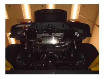
**Step 4.** Complete the installation by attaching the Muffler Assembly onto the Resonator Assemblies using the supplied 3.00" clamps. Fit the hangers into the rubber insulators and re-attach the vaccum lines
