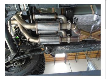
**Step 3.** Next install the Resonator Assemblies using the supplied V-Band clamps. Fit the hanger on the driver side assembly into the rubber insualtor.
