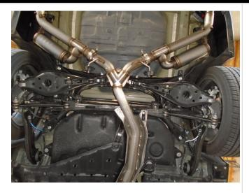
**Step 4.** Install the Muffler Assemblies in a similar fashion using the supplied 2.50" V-clamps and fitting the hangers into the insulators.
