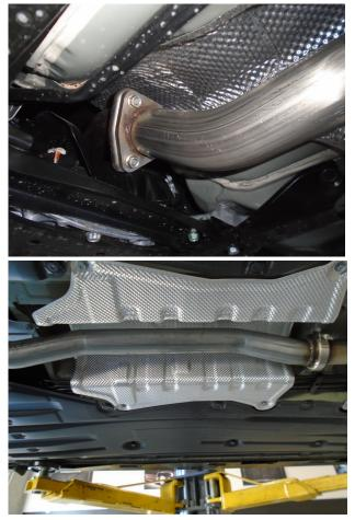
**Step 2.** Install your new system by first mounting the Inlet Pipe Assembly to the outlet flange using the OE fasteners and then attaching the MidPipe to the Inlet pipe using a supplied 2.50" V-clamp. leave clamps and fasteners loose until install is complete
