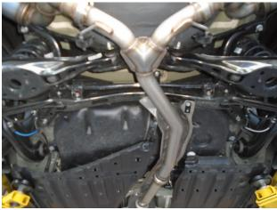
**Step 3**. Next, using the supplied 2.50" V-Clamp loosely attach the Y-Pipe Assembly to the Mid Pipe Assembly and attach the hanger to the rubber insulator.
