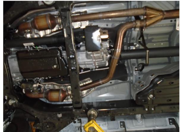
**Step 2:** Begin Installation of the new MagnaFlow system by attaching Passenger side Inlet Assembly using the OE fasteners and gaskets. Next install the Driver side in a similar fashion (using OE fasteners) and using a supplied 2.50" clamp attach it to the Passenger side inlet. (Leave all clamps and fasteners loose until final adjustment for fit.)
