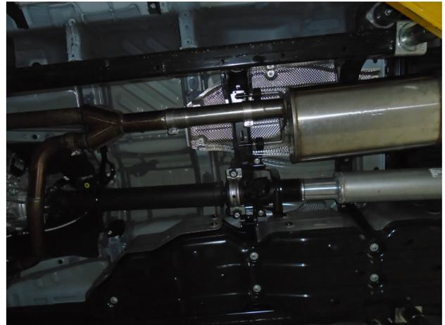
**Step 3:** At this point if you are installing the MagnaFlow exhaust system on a Long Bed vehicle you will need to add the 15" Extension Pipe using the supplied 3.00" clamp. (The short bed does not require this pipe).
