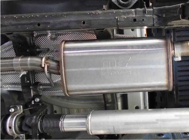
**Step 4:** Attach the Muffler Assembly by fitting it to the Extension Pipe (or Inlet Assembly) using the supplied 3.00" clamp and fitting the hangers into the rubber insulators.
