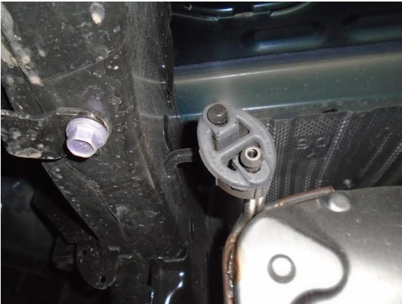
**Step 1:** To remove the OE exhaust system, loosen fasteners at the inlet flanges (2) where they connect to the catalytic converters. Working front to rear disengage the hangers from the rubber insulators, remove the remaining fasteners at flange junctions and drop the system. (Retain the Inlet fasteners, gaskets and rubber insulators as they will be used to install your new system.)
