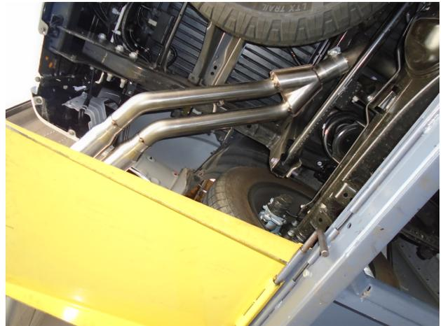
**Step 6:** Finish the installation by attaching the Tail Pipe Assembly to the Over Axle Pipe using the supplied 3.00" clamp and fitting the hanger into the rubber insulator.
