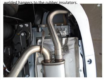
**Step 6.** Install the Tail Pipe Assemblies by locating the outlets through the rear valance tip. Then loosely secure to the Muffler Assembly outlet using the supplied clamps. Engage he welded hangers to the rubber insulators.
