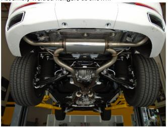
**Step 8.** Once a final position has been chosen for the new exhaust system, evenly tighten all clamps from front to rear using the torque specifications on page one of these instructions. Inspect all fasteners after 25-50 miles of operation and re-tighten if necessary.
