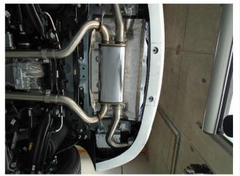
**Step 5.** Install the Muffler Assembly by loosely attaching the two inlet pipes to the X-Pipe Assembly outlet pipes using the supplied clamps. Engage the
