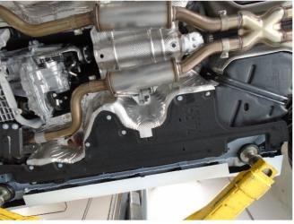
**Step 3.** Begin installing the new system by loosely attaching the Resonator Assembly inlets to the catalytic convert outlets using the supplied clamps. Engage the welded hangers to the rubber insulators.
