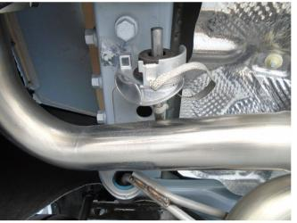
**Step 7.** Finally, clip the grounding leads to the Tail Pipe Assembly welded hangers as shown.
