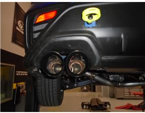
**Step 6.** Once a final position has been chosen for the new exhaust system, evenly tighten all clamps from front to rear using the torque specification on page one of these instructions. Inspect all flasteners after 25-50 miles of operation. Re-tighten if necessary.
