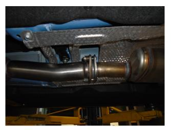
**Step 3**. Begin installation of the new system by fastening the Inlet Pipe Assembly to the outlet of the catalytic converter using the OEM hardware..
