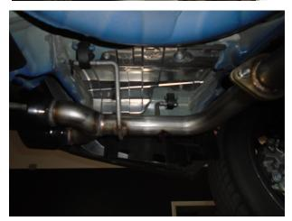
**Step 5.** Next loosely install both Tail Pipes by bolting the inlets flanges to the Y-Pipe Assembly using the OEM hardware and supplied gaskets. Insert all welded hangers into the OEM rubber insulators.
