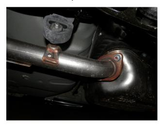
**Step 2.** With the system supported disengage all welded hangers from the rubber isolators. The OEM exhaust system may now be removed.
