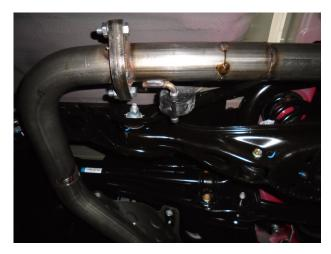
**Step 5**: Loosely attach the Muffler Assembly flange to the Mid-Pipe Assembly. Secure with the supplied gaskets and hardware. Engage welded hangers to rubber insulators.
