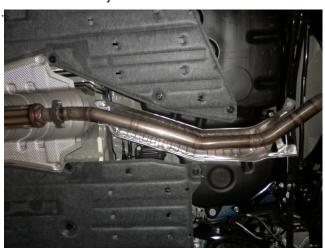
**Step 4.** Next attach the Mid-Pipe Assembly to the Inlet Resonator Assembly by fastening the flanges using the supplied gasket and hardware.
