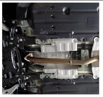
**Step 2:** MagnaFlow supplies this kit with a Delete pipe, it can be used in place of the Resonator for a more aggressive sound.
