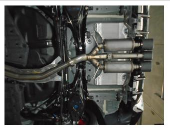
**Step 4:** Finish by loosely installing the Mid Pipe and Muffler Assembly using the supplied clamp and fitting the hangers into the rubber insulators.
