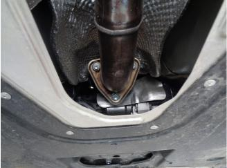
**Step 1:** To remove the OEM system first unbolt and remove the cross member at the inlet. Next, unbolt the inlet pipe at the catalytic converter flange junctions. Working front to rear disengage all welded hangers from the rubber insulators. The OE exhaust system can now be removed in one piece. Be sure to retain all mounting hardware as it will be needed to install your new MagnaFlow system
