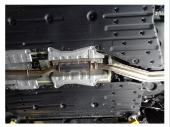
**Step 3:** Next, loosely fasten either the Resonator Assembly or the Delete Pipe to the Inlet Assembly using the supplied clamps.
