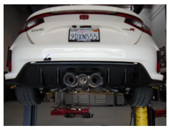
**Step 5:** Once a final position has been chosen for the new exhaust system, evenly tighten all clamps from front to rear using the torque specifications on page one of these instructions. Inspect all fasteners after 25-50 miles for operation and re-tighten if necessary.
