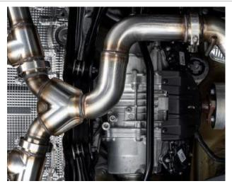
**Step 6**: Next loosely install the Y-Pipe Assembly using the supplied V-Band clamp.
