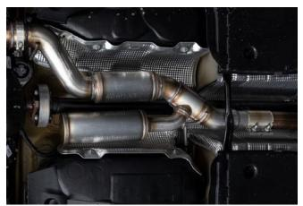
**Step 5.** Loosely attach the Inlet Pipe Assembly to the OEM slip clamp. Engage the welded hangers to the rubber insulators.
