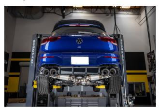
**Step 8:** Once a final position has been chosen for the new exhaust system, evenly tighten all clamps from front to rear using the torque specifications on page one of these instructions. Inspect all fasteners after 25-50 miles for operation and re-tighten if necessary.
