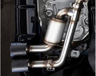
**Step 7.** Loosely install the Resonator Assemblies using the supplied V-Band clamp. Attach the welded hangers to the rubber insulators. Re-attach both electrical connectors to the exhaust valve motors.
