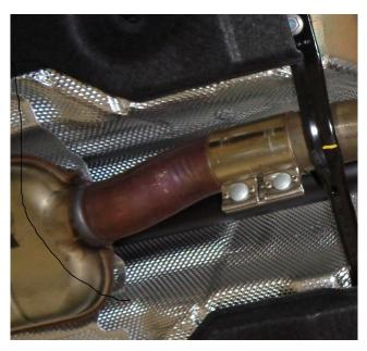
**Step 2.** Begin removal of the OEM system by loosening the slip clamp at the vehicles exhaust inlet. Working front to rear disengage all welded hangers from the rubber insulators. Be sure to retain all mounting hardware as it will be needed to mount your new MAGNAFLOW exhaust.
