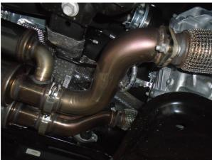
**Step 7:** Begin installation of the MagnaFlow system by attaching the inlet pipe assemblies using the OE fasteners and fitting the hangers into the rubber insulators.
