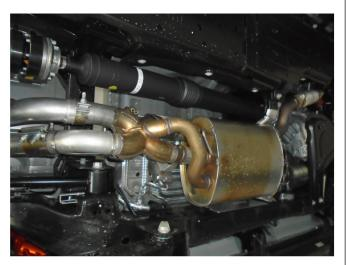
**Step 2:** Next loosen the clamps on both pipes that exit the X-Pipe. With the exhaust supported working front to back remove the OE exhaust system. You are now ready to install your new MAGNAFLOW exhaust system
