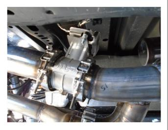
**Step 10:** Next install the valves using the supplied clamps and fit the electrical plugs.
