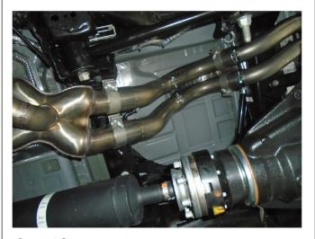
**Step 12:** Attach the Driver and Passenger side over axle assemblies to the X-Pipe using the supplied 2.50" Torca clamps and fitting the hanger into rubber insulator.
