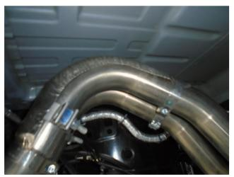
**Step 6:** Before beginning the exhaust installation the heatshields from the OE over axle pipes need to be removed and transferred to the MagnaFlow system. Cut the retaining straps securing the heatshield and move them over to the MagnaFlow Over Axle pipes (2) and secure using the supplied worm drive clamps.
