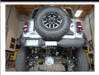
**Step 14:** Once a final position has been chosen for the new exhaust system, evenly tighten all clamps and fasteneners, from front to rear, using the torque specifications on page one of the instructions. Inspect all fasteners after 25-50 miles of operation and re-tighten if necessary.
