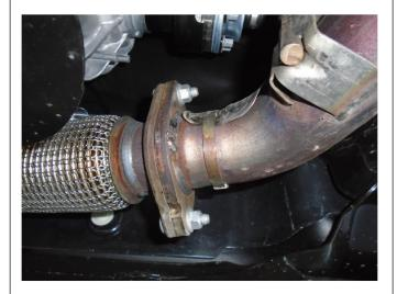
**Step 1:** Begin removal of your OE system by first loosening the fasteners from the front 2 bolt flanges (2) and un-plugging the electrical connections to the valves. Disengage all welded hangers from the rubber insulators. Do not damage the fasteners, heatshields (on the overaxle pipes) and rubber insulators as they will be used to install your new system.
