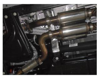
**Step 8:** Loosely install the two Muffler/NDT Resonator Assemblies using the supplied clamps. Orientate as shown
