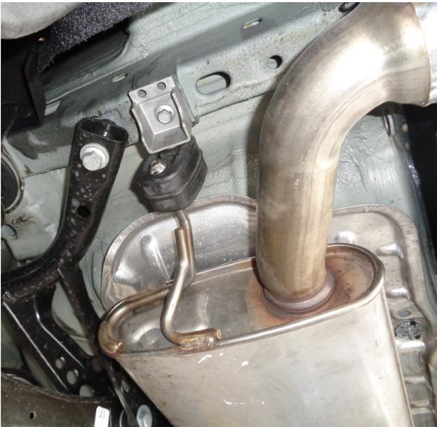
Step 2. Next, Disengage all welded hangers from the rubber insulators. The exhaust system can now be removed. Retain all fasteners and insulators as they will be needed to mount your new MAGNAFLOW system.
