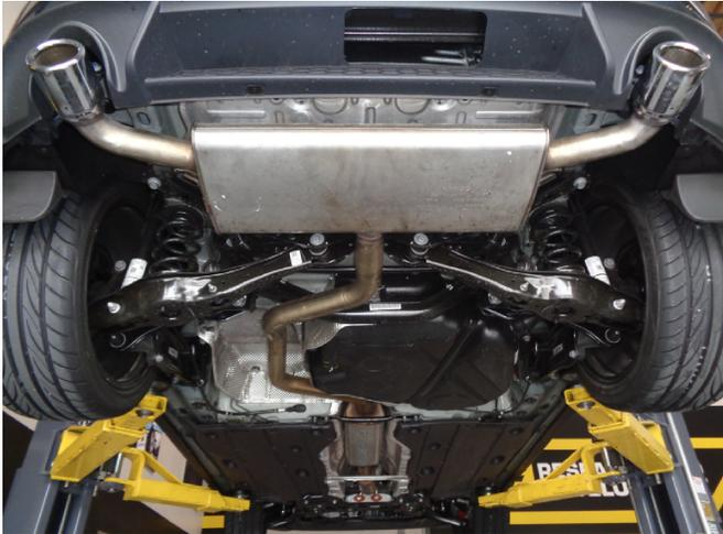
Step 1. Remove the OEM system by first unbolting the two nuts at the slip, attaching the stock inlet pipe to the catalytic converter.
