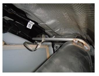
**Step 6.** Finally, clip the grounding leads to the Tail Pipe Assembly welded hangers as shown.
