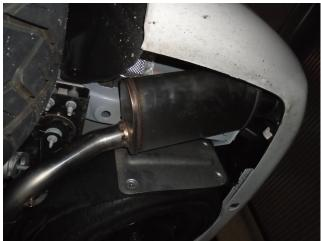
**Step 5.** Install the Muffler Assemblies by loosely attaching the inlet pipes to the X-Pipe Assembly outlet pipes using the supplied clamps. Engage the welded hangers to the rubber insulators.
