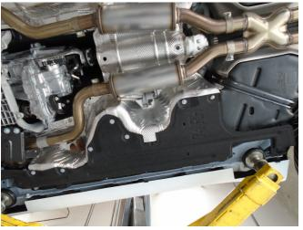
**Step 3.** Begin installing the new system by loosely attaching the Resonator Assembly inlets to the catalytic convert outlets using the supplied clamps. Engage the welded hangers to the rubber insulators.
