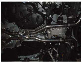
**Step 4.** Install the X-Pipe Assembly by loosely securing both inlets to the Resonator Assembly outlets using the supplied clamps. The longer pipe should be oriented on the drivers side.
