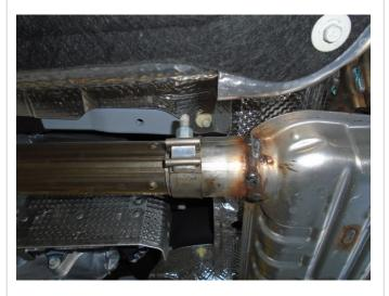
**Step 2.** Loosen the two clamps attaching the muffler assembly to the catalytic converter outlets. Disengage all welded hangers from the rubber insulator, do not discard as they will be needed to install the new MAGNAFLOW system. The OEM system can now be removed.
