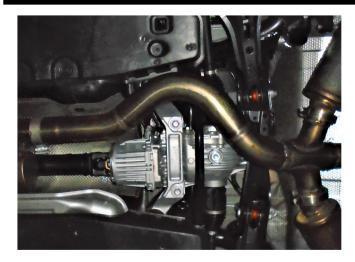
**Step 4:** Next, attach the Center Tailpipe Assembly to the Resonator using the supplied 3.00 Clamp. Keep this section supported until the installation is complete.
