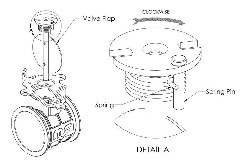
Before installing the OE Valve Motor to the MagnaFlow valve it is very important to have the valve flap oriented correctly.
