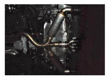
**Step 5:** Finish the installation by fitting the Driver and Passenger Side Muffler Assemblies onto the Center Tailpipe Assembly using the supplied Band Clamps and fitting the hangers into the rubber insulators. You can now plug the connector back into the valve motor.
