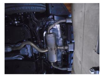
**Step 1:** To remove the OE exhaust begin by unplugging the valve motor at the center tailpipe then un-fasten the hardware at the flange. While supporting the exhaust extract the hangers from the rubber insulators (retain the fasteners and rubber insulators as they will be re-used).
