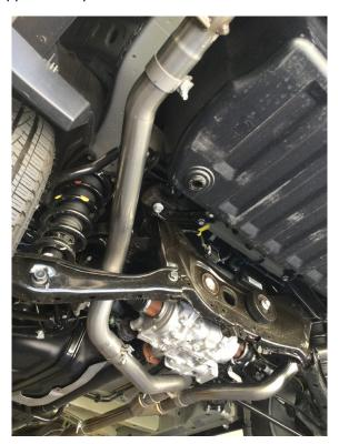
**Step 4:** Install the Crossover Pipe Assembly in a similar fashion using the supplied clamp and engaging the welded hanger to the rubber insulator.
