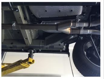
**Step 3:** Next loosely fasten the Y-Pipe Assembly inlet to the outlet of the Muffler Assembly using the supplied clamp.
