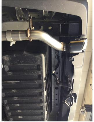
**Step 5:** Finish by installing the Extension and Tailpipe Assemblies using the supplied clamps and by fitting the hangers into the rubber insulators.
