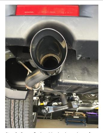
**Step 6:** Once a final position has been chosen for the new exhaust system, evenly tighten all clamps from front to rear using the torque specifications on page one of these instructions. Inspect all fasteners after 25-50 miles of operation and retighten if necessary.
