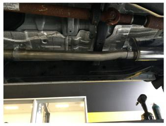
**Step 3.** Next loosely attach the Inlet Extension Pipe Assembly to the Inlet Pipe Assembly using the supplied clamp. Engage the welded hanger to the rubber insulator.
