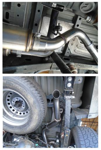
**Step 5.** Loosely install the Over Axle Pipe and Tail Pipe Assemblies locating the welded hangers to the rubber insulators and secure using the supplied clamps.
