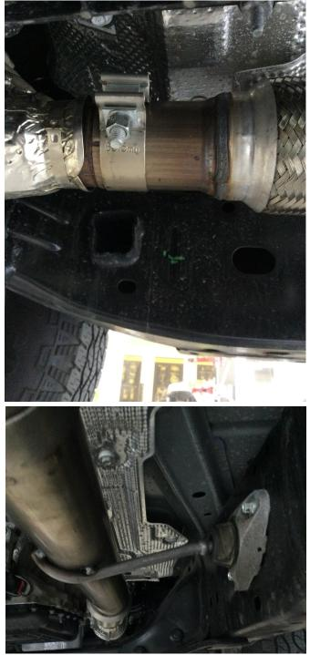
**Step 2.** To begin, loosely fasten the Inlet pipe assembly to the outlet of the OE catalytic converter using the Supplied clamp. Engage the welded hanger into the rubber insulator (Leave all clamps and fasteners loose for final adjustment of the complete system.)
