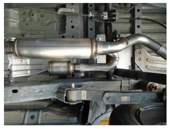
**Step 4.** The Muffler is configurable to suit your sound and performance preference. Use the chart below as a guide. Install the Muffler inlet to the extension pipe outlet with the supplied clamp.
