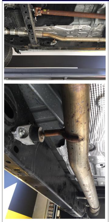
**Step 1.** To remove the OEM exhaust system disengage the welded hangers from the rubber insulators and remove the tailpipe assy. Unfasten the clamp attaching the OEM inlet pipe assembly to the catalytic converter. Do not damage or discard the rubber insulators as they will be re-used to mount the new system. Disengage the inlet pipe assembly hanger and remove the exhaust from the vehicle.
