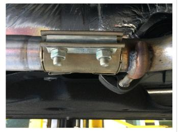
**Step 2:** Begin removing the OEM exhaust system by loosening the clamps located rearward of the catalytic converter. Next working front to rear extract the hangers from the rubber insulators and remove the OEM system. Retain insulators and clamps as they will be used to install the new system. Remove actuators from OEM exhaust valve and install on new rear muffler assemblies valves. Reuse OEM fasteners. replacement heat shields and springs are supplied.
