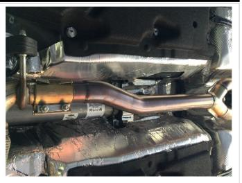
**Step 3:** Begin installation of the new system by loosely attaching the Y-Pipe Assembly to the catalytic converter outlet using the OEM clamps. Leave all clamps loose until final adjustment.
