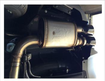
**Step 5:** Install the Muffler Assemblies to the Mid Pipe Assemblies using the supplied clamps. Locate the welded hangers to the rubber insulators.
