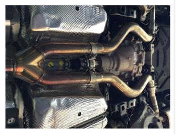
**Step 4:** Next attach both Mid Pipe Assemblies to the Y-Pipe Assembly using the supplied clamps. Locate the welded hangers to the rubber insulators.
