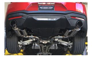
**Step 5:** Once a final position has been chosen for the new exhaust system, evenly tighten all clamps from front to rear using the torque specifications on page one of these instructions. Inspect all fasteners after 25-50 miles for operation and re-tighten if necessary.
