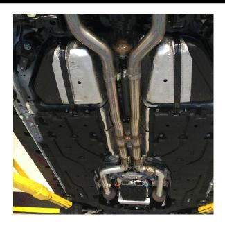
**Step 2:** Begin installation of the new system by loosely attaching the H-Pipe Assembly to the outlets using the OEM clamps. Leave all clamps loose until final adjustment.
