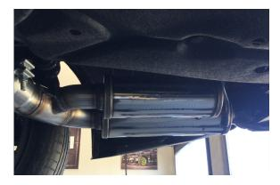
**Step 4:** Finish the initial installation by fitting the Muffler Assemblies onto the Mid pipe Assemblies using the supplied 3.00" clamps and inserting the hangers into the rubber insulators.
