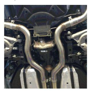
**Step 3:** Next attach the Mid Pipe Assemblies to the H-Pipe using the supplied 3.00" clamps and fitting the hangers into the rubber insulators.
