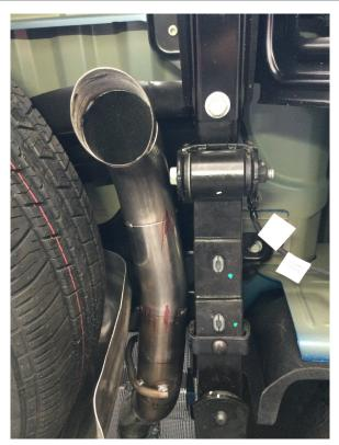
**Step 7:** Installing the Tail Pipe to the Over Axle Pipe outlet using the supplied clamp. Engage the hanger to the OE rubber insulator. Clearances are very tight, make sure there is adequate room after tightening.
