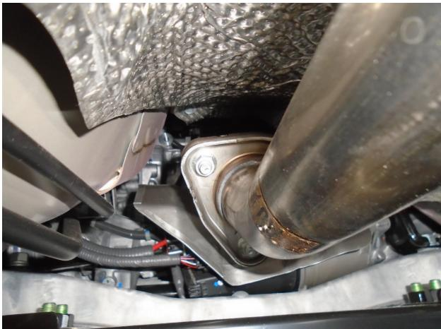
**Step 1.** Begin removal of the OEM exhaust system by unbolting the inlet flange attaching the exhaust to the catalytic converter. Do not discard or damage the OEM fasteners or rubber insulators as they will be used to install the new system
