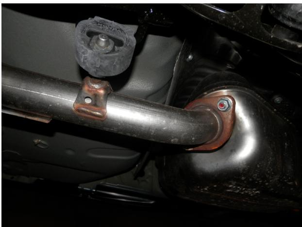
**Step 2.** Unbolt the drivers side OEM muffler assembly at the flange junction. Disengage all welded hangers from the rubber isolators. The OEM exhaust system may now be removed.
