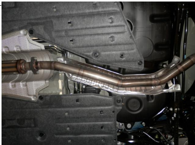
**Step 4.** Next attach the Y-Pipe Assembly to the Inlet Resonator Assembly by fastening the flanges using the supplied gasket and hardware.
