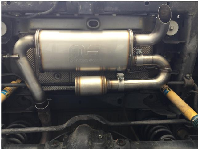
Step 2. Next, slide the MagnaFlow axle-back into the OE over-axle pipe and loosely clamp to hold in place. Then slide the hangers into the factory rubber insulators. Next attach the NDT resonator and clamp in place.
