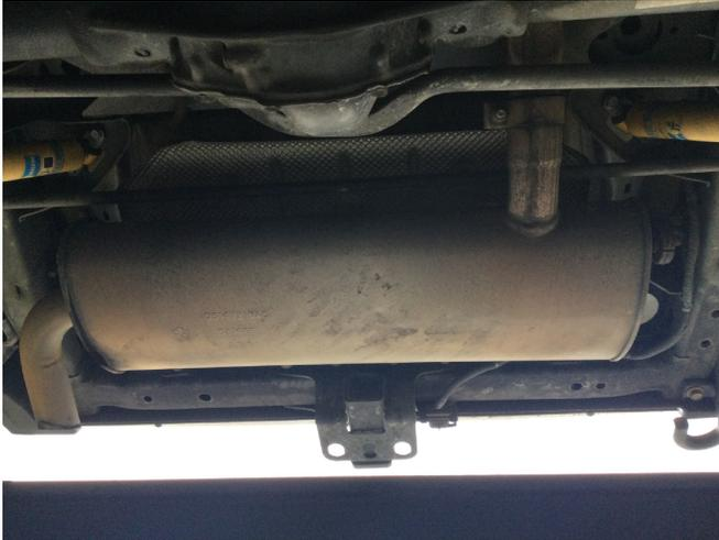
Step 1. Remove the OEM system by loosening the over-axle TORCA clamp. Then disconnect the OE rubber hangers and remove the OE muffler.
