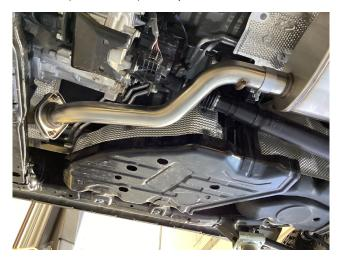
**Step 2**: Begin Installation of the new MagnaFlow system by attaching Inlet Assembly using the OE fasteners and supplied gasket. (Leave all clamps and fasteners loose until final adjustment for fit.)
