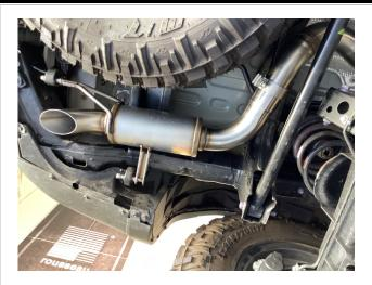
**Step 5**: Install the rear Muffler Assembly to the Over Axle Pipe fitting the hanger into the rubber Insulator.
