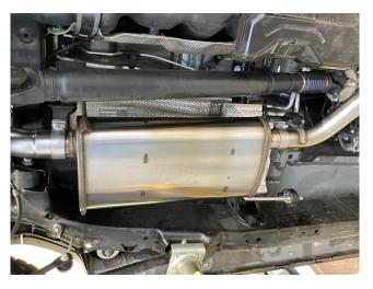
**Step 3:** Next install the Muffler Assembly using the supplied 2.50" clamp and fit the hangers into the rubber insulators.
