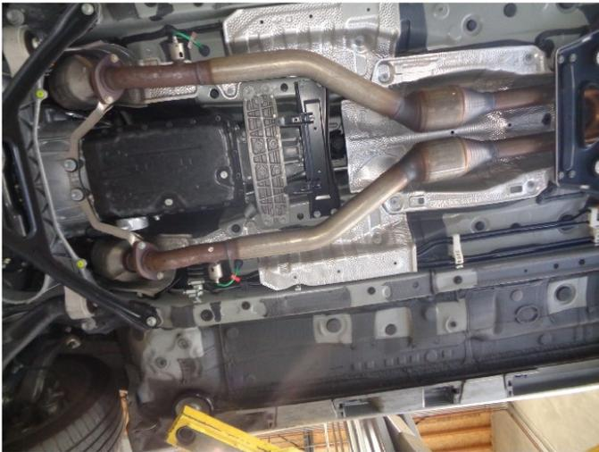
2. Remove the two O2 sensors and unbolt the exhaust inlet flanges at the catalytic converters. The center section may now be removed. Be sure to retain all mounting hardware as it will be needed to install your new MAGNAFLOW system.
