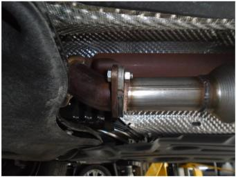
**Step 5.** Install the supplied clamp onto new MagnaFlow converter end and install over cut pipe on vehicle. Bolt the converter flange into place using the supplied fasteners.
