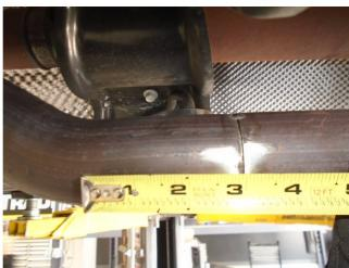
**Step 1.** Begin by measuring 3" from the tangent of the pipe bend as shown, and mark.
