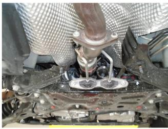
**Step 2.** Cut pipe at marked location. Loosen fasteners from inlet flange and remove converter. Clean and deburr cut pipe remaining on vehicle.
