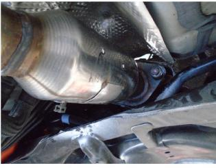
**Step 5.** Install the supplied clamp onto new MagnaFlow converter end and install over cut pipe on vehicle. Bolt converter flange into place using the OE fasteners.
